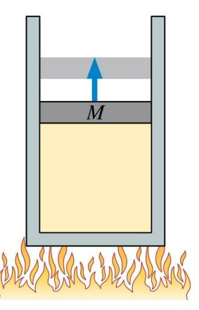
A cylinder of gas has a frictionless but tightly sealed piston of mass *M*. A small flame heats the cylinder, causing the piston to slowly move upward. For the gas inside the cylinder, what kind of process is this?
