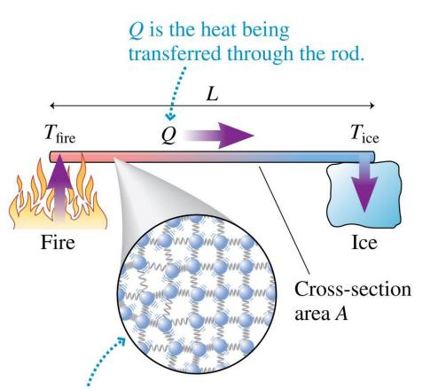
The particles on the left side of the rod are vibrating more vigorously than the particles on the right. The particles on the left transfer energy to the particles on the right via the bonds connecting them.
