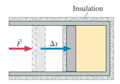
A steady force pushes in the piston of a well-insulated cylinder. In this process, the temperature of the gas
