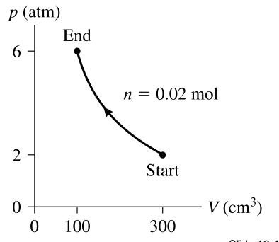
A sample of gas is in a cylinder with a moveable piston. The force on the piston can be varied, altering the pressure and volume. A sample of gas is taken from an initial state to a final state following a curve on the pV diagram shown. The final temperature is
