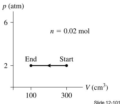
A steady force pushes in the piston of a well-insulated cylinder. In this process, the temperature of the gas
