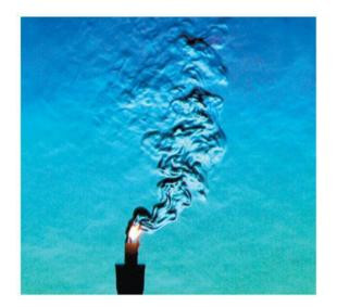
This special photograph shows air currents near a warm glass of water. Air near the glass is warmed and rises, taking thermal energy with it in a process known as *convection*. **Energy is transferred by the bulk motion of molecules with high thermal energy.**
