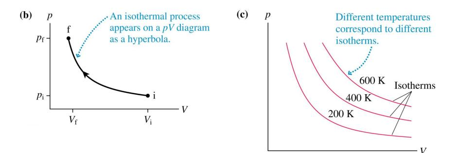
A sample of gas is in a cylinder with a moveable piston. The force on the piston can be varied, altering the pressure and volume. A sample of gas is taken from an initial state to a final state following a curve on the pV diagram shown. The final temperature is
