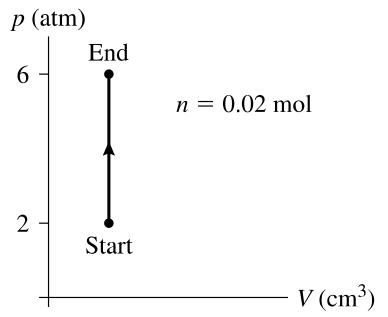
A sample of gas is in a cylinder with a moveable piston. The force on the piston can be varied, altering the pressure and volume. A sample of gas is taken from an initial state to a final state following a curve on the pV diagram shown. The final temperature is
