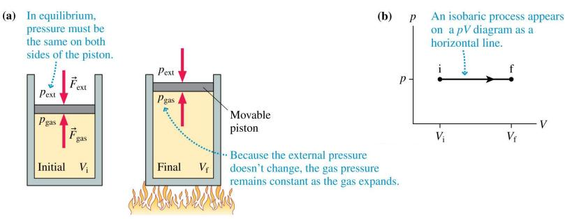
A sample of gas is in a cylinder with a moveable piston. The force on the piston can be varied, altering the pressure and volume. A sample of gas is taken from an initial state to a final state following a curve on the pV diagram shown. The final temperature is
