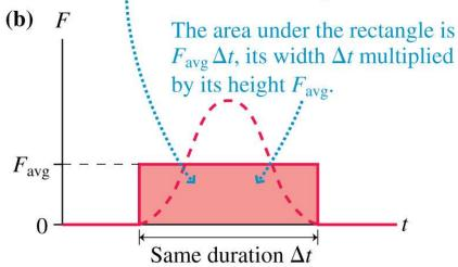
impulse J = area under the force curve  $= F_{\text{avg}} \Delta t$
