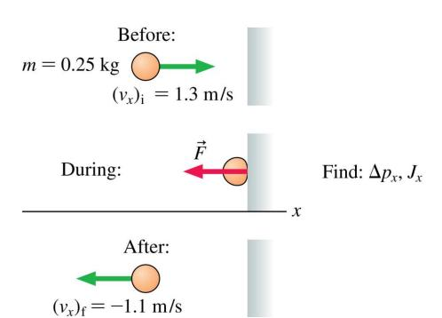
PREPARE A visual overview of the ball bouncing is shown in FIGURE 9.8. This is a new kind of visual overview, one in which we show the situation "before" and "after" the interaction. We'll have more to say about beforeand-after pictures in the next section. The ball is moving along
