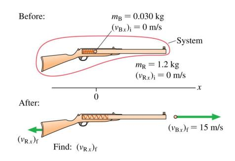
FIGURE 9.20 shows a visual overview before and after the ball is fired. We'll assume the ball is fired in the +x-direction.
