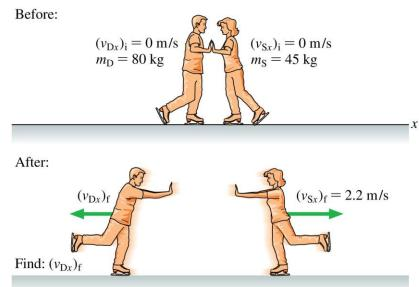
$$m_{S}(v_{Sx})_{f} + m_{D}(v_{Dx})_{f} = m_{S}(v_{Sx})_{i} + m_{D}(v_{Dx})_{i} = 0$$
