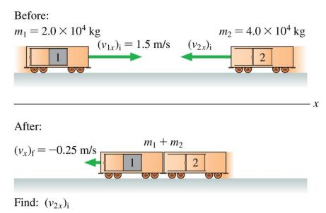
car has an initial speed of 1.5 m/s; the collision causes it to reverse direction at 0.25 m/s. What was the initial speed of the heavier car?
