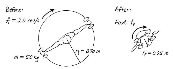
**PREPARE** There is no external torque acting on the system consisting of the skater and the weights, so their angular momentum is conserved. FIGURE 9.29 shows a before-and-after visual overview, as seen from above.
