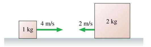
The two boxes are sliding along a frictionless surface. They collide and stick together. Afterward, the velocity of the two boxes is
