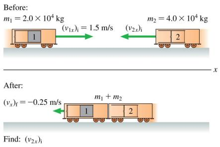
**ASSESS** The key step in solving inelastic collision problems is that both objects move after the collision with the same velocity. You should thus choose a single symbol (here,  $(v_x)_f$ ) for this common velocity.
