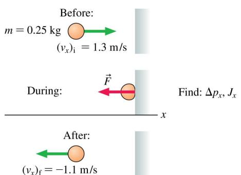
$$\Delta p_x = (p_x)_f - (p_x)_i = (-0.275 \text{ kg} \cdot \text{m/s}) - (0.325 \text{ kg} \cdot \text{m/s})$$
