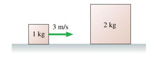
The 1-kg box is sliding along a frictionless surface. It collides with and sticks to the 2-kg box. Afterward, the speed of the two boxes is
