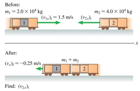
FIGURE 9.23 shows a visual overview. We've chosen to let the  $2.0 \times 10^4$  kg car (car 1) start out moving to the right, so  $(v_{1x})_i$  is a positive 1.5 m/s. The cars move to the left after the collision, so their common final velocity is  $(v_x)_f = -0.25$  m/s. You can see that velocity  $(v_{2x})_i$  must be negative in order to "turn around" both cars.
