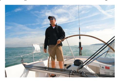
• You'll see that torque depends on how hard you push and also on *where* you push. A push far from the axle gives a large torque.
